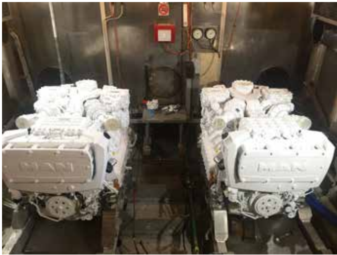
Both engines in position and mounted to the vessel bearers and prop shaft. Now for the connection of the raw water, fuel system, electrics and exhaust.
