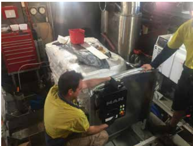
Both engines in position and mounted to the vessel bearers and prop shaft. Now for the connection of the raw water, fuel system, electrics and exhaust.
