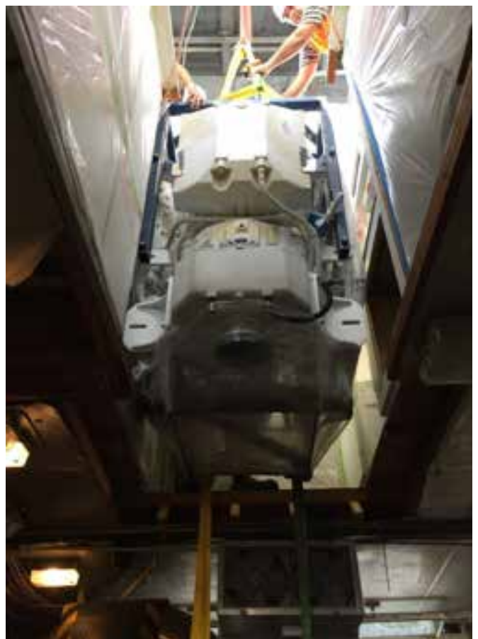
With mm's to spare we lowered the engine into the vessel.
