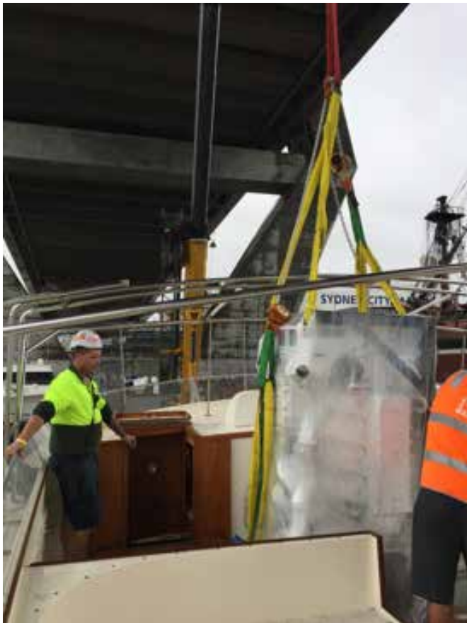
With mm's to spare we lowered the engine into the vessel.
