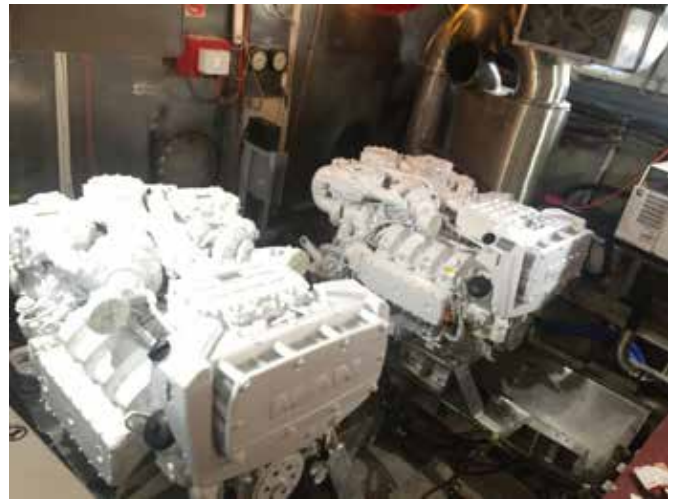
Both engines in position and mounted to the vessel bearers and prop shaft. Now for the connection of the raw water, fuel system, electrics and exhaust.
