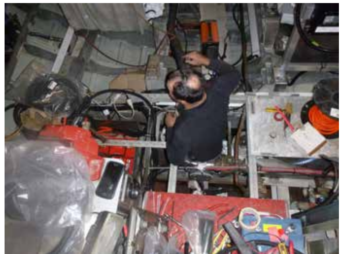
Both engines in position and mounted to the vessel bearers and prop shaft. Now for the connection of the raw water, fuel system, electrics and exhaust.
